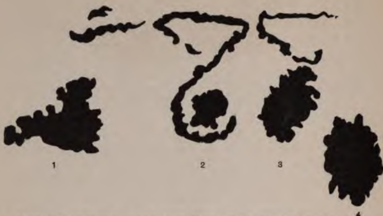
CONTACTS OF 33-INCH WORN CAST IRON WHEEL UNDER GONDOLA CAR. WEIGHT ON WHEEL, 14,575 LBS.
